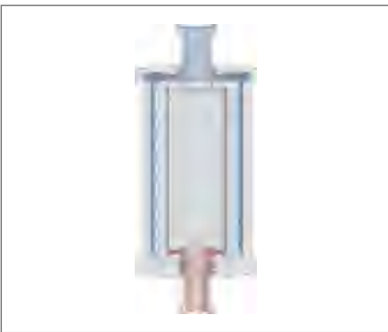
Fig. 12: Sartobind 150 mL capsule cross section displays small upstream and downstream channels
