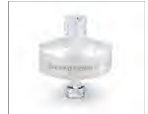
Fig. 7: Sartobind Protein A 2 mL runs at 10 mL/min with a dynamic binding of 10–15 mg IgG per unit
