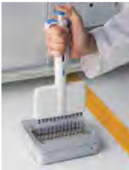
Detailed view: pipetting into the weighing tubes
