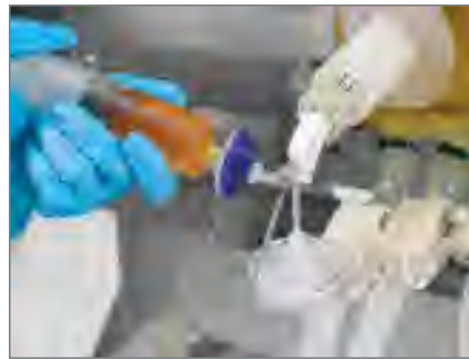
Figure 3: Calibration of the single-use pH probe
